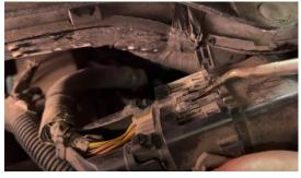
Pulling the junction box toward the engine with your left hand, insert a flathead screwdriver or pick behind the junction box from the right side and under the tab lock which is dead center. Slightly lift the tab by pulling toward the radiator. Once the tab is released, with your left hand pull junction toward the engine to disconnect.
